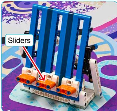
Rotate the sound mixer's reset lever completely outward and lower the sliders down completely.
