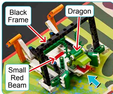
Make sure the small red beam is horizontal and push the dragon completely in.
